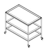
1. Attach End Frames to Crossbar ×4 with M8×25 CSK Machine Screw ×16
