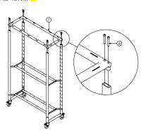
**5.** Place (x2) Shelf Panels on the fixed Crossbars at the base and middle of the unit. Angle the Panels during insertion, as shown.
