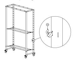
**6a.** Shelf Panels can also be angled by placing rear Shelf Brackets one row higher than the front brackets.
