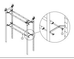
**4.** Flip the frame assembly and attatch the Top Frame with M8x50 Special Socket Screws.  $\triangle$  Tighten to 40NM  $\triangle$
