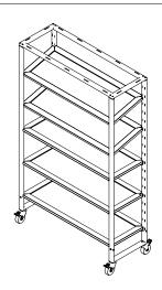
1. With the End Frame upside down, attach (x2) Castor Wheels with M12x30 & M12 Washer. Ensure castors are locked before attaching.  $\triangle$  Tighten to 100NM  $\triangle$
