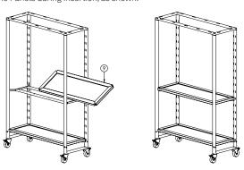
**6.** To fit Shelf Panels at other heights, insert x4 Shelf Brackets in to the inward column of frame slots at required height.
