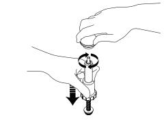
6. Install the cylinder 1 onto the valve body.
