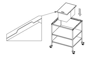
2. Carefully slide the Ice Well to the desired side of the trolley, ensuring it makes contact with the bumpers on the vertical edge of the top frame.
