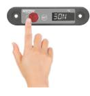
Press **Key Up** and hold for 3 seconds to turn unit on or off.
