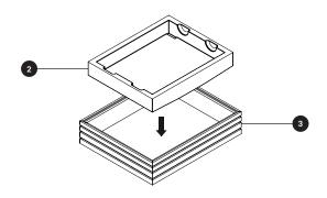
**2b.** For 1.1 trays, position 2 Insulating Tray Liners as shown:
